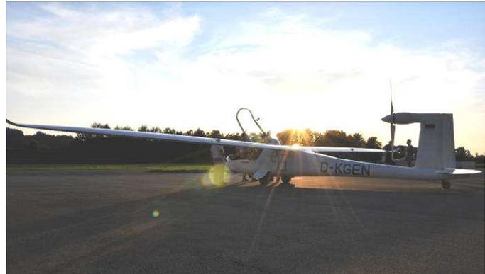
Due to that and also because of the fact that electric drive systems can indeed be activated, i.e. “switched on”, but at the same time not necessarily need to move, rotate or even make a sound, there is a considerable risk that there are people, animals or objects in the propeller disk area and that they can be injured or damaged accidentally during the run-up of the propeller. This risk is especially high for recreational aircraft which are not always operated from strictly guarded airfields.
