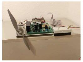
The *ePropeller Safety Device* is a concept to avoid such accidents without adding extra weight or extra components to the aircraft. Using the motors own sensors and microcontrollers, the propeller disk area is checked for obstacles during the run-up phase. For a short period, *eSD* operates the drive system in a protected mode, switching automatically to the normal operation mode after the disk area is detected clear.
